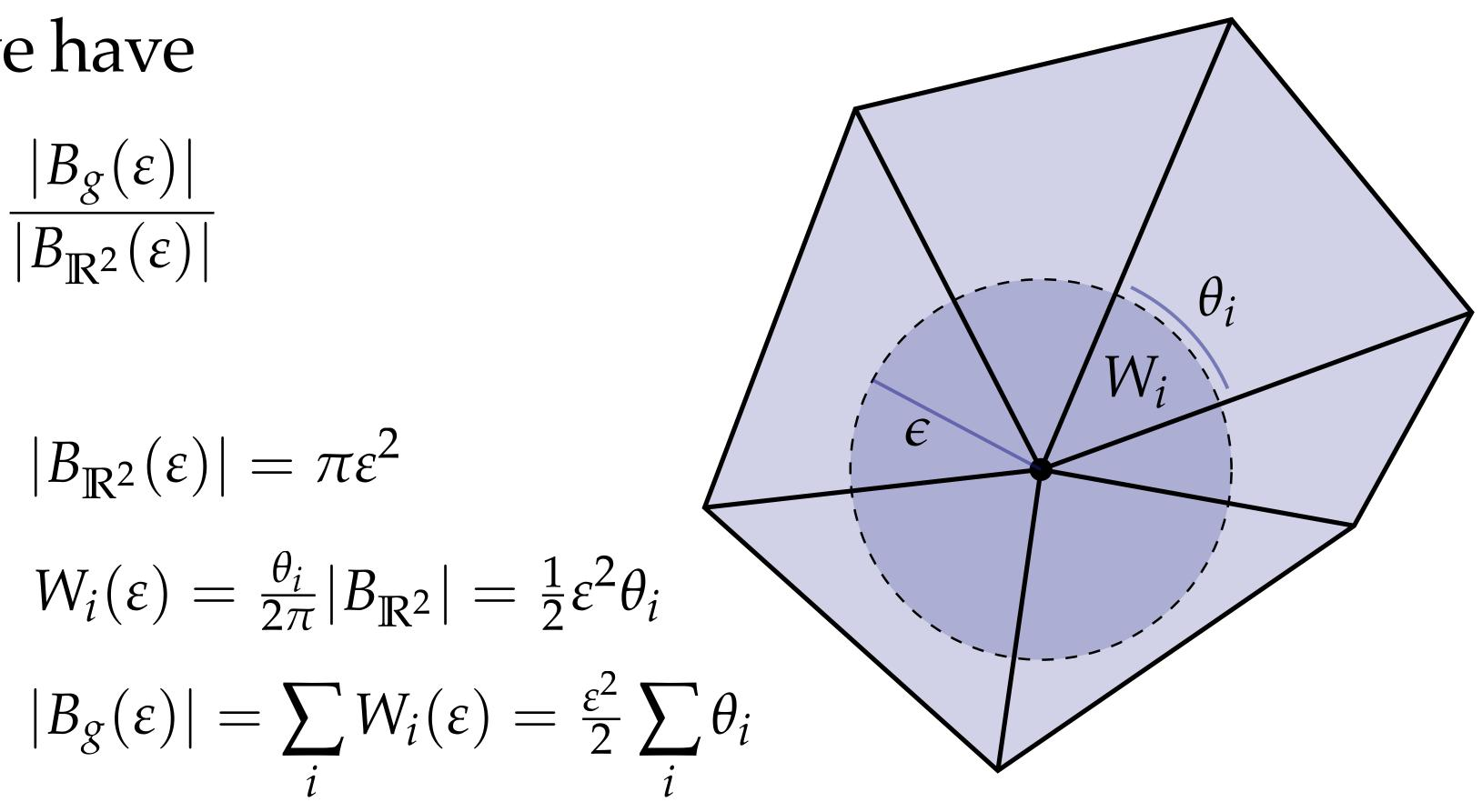
Angle defect is integrated curvature
