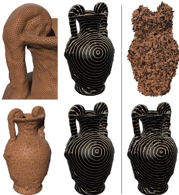
Figure 19. Tests of robustness. Left: our smoothed distance ( m = 10^4 ) appears similar on meshes of different resolution. Right: even for meshes with severe noise (top) we recover a good approximation of the distance function on the original surface (bottom, visualized on noise-free mesh).
