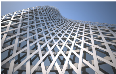
Figure 45: A 3-web of curves which are geodesic within tolerance, is the basis of this weaving design manufacturable by bending wooden panels. The geodesic property, if rigidly enforced, is a global property of a curve — see also Fig. 13.
