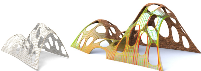
Figure 49: Optimizing surfaces for the self-supporting property. Left : Cutting holes in a self-supporting surface will destroy the self-supporting property. Right : Vouga et al. [109] show how to find the closest self-supporting surface. The image also shows the fictitious thrust network of forces which by Heyman’s “safe theorem” guarantees stability.
