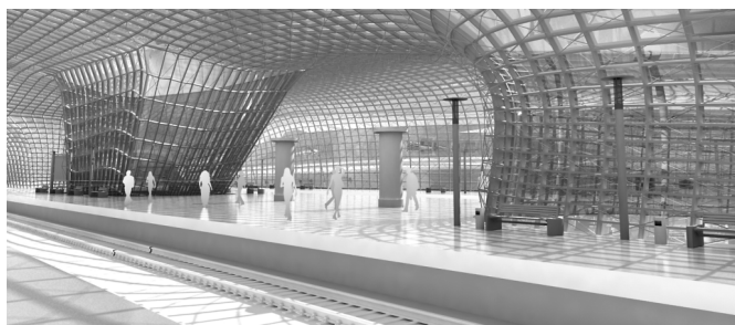
Figure 7. Discrete parameterized surfaces play a role in architectural geometry, where special incidence relationships on quadrilaterals translate to manufacturing constraints like zero nodal torsion, or offset surfaces of constant thickness. Here a curvature line parameterized surface discretized by a conical net is used in the design of a railway station.
