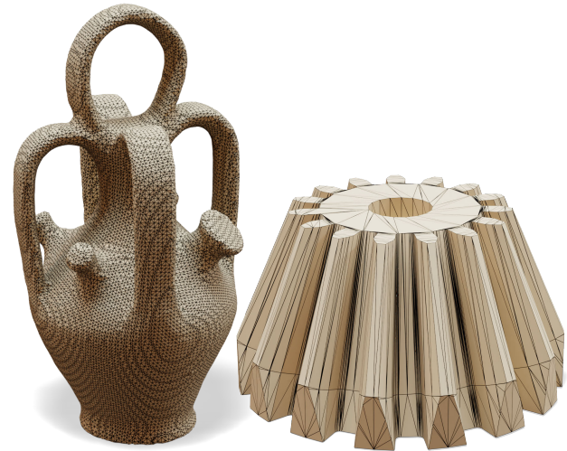
Fig. 4. An intrinsic triangulation exactly preserves the input geometry, while changing the mesh connectivity. Hence, if the input mesh gives an exact description of the geometry (as with the CAD model at right), it will not be corrupted; if the input exhibits noise or approximation error (as with the marching cubes approximation at left), these errors will get neither better nor worse.
